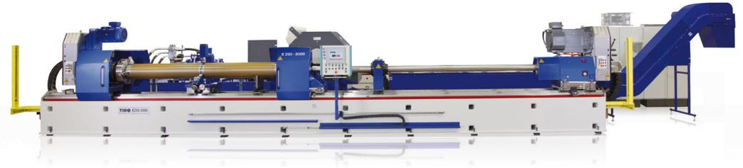
The TIBO B250 will give Hone-All a 250mm diameter capacity with 3.2m machining length whilst the TIBO B80 will provide 80mm diameter machining with a 3.2m length.
