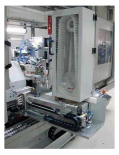
A combination of several of the above-mentioned automation is also possible. For example, a robot that places the components on a conveyor or removes them from it and a magazine for automatic tool changes in BTA-deep drilling machines, or a component magazine for small components on the machine with an integrated gripper for inserting the components on the workpiece pre-centring device in a multi-spindle gun-drilling machine.
